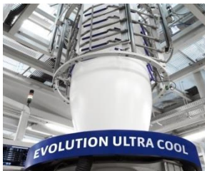
Film production on blown film line
